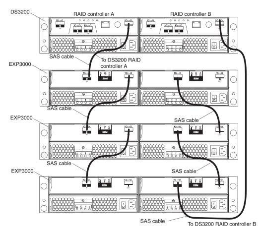
Figure 22. One dual-controller DS3200 and three storage expansion enclosures
